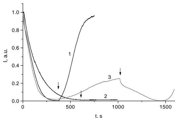
Fig. 3. Recording and self-erasure. Arrows point switch off the excitation. (1) – nonbaked sample, (2) – baked sample, (3) excitation for more than  $180^\circ$  anisotropic phase delay
