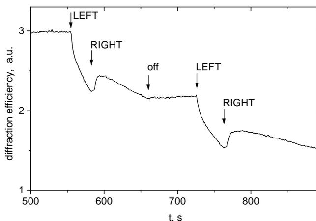
Fig. 4. Erasure of the recorded grating alternatively with left and right circularly polarized beam.
