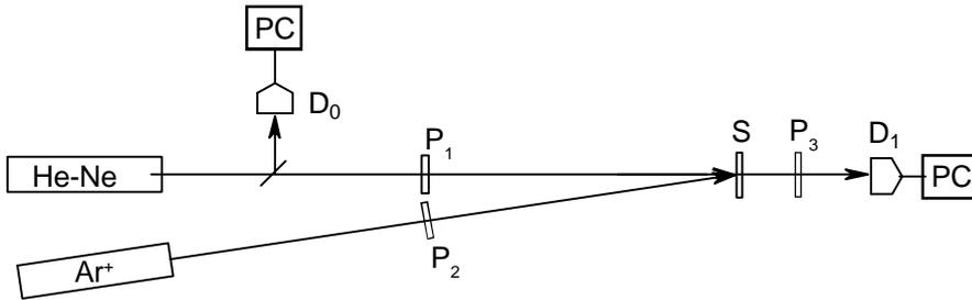
Fig. 2. Experimental Setup. P<sub>1</sub> – polarizers, D<sub>1</sub> – photo-detectors, S – sample
